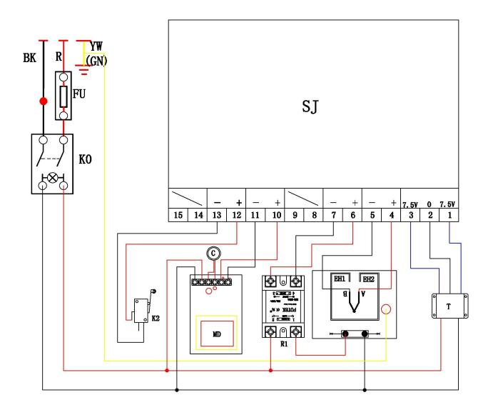
Ko.: Power switch C: Electromagnet K2: Limit Switch
